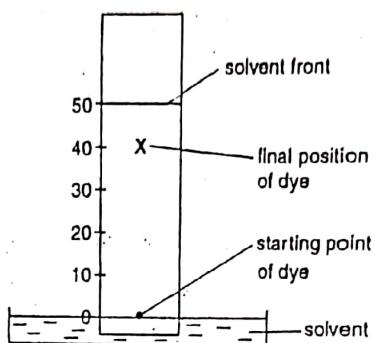
which fraction shows the R<sub>f</sub> value for the dye?
